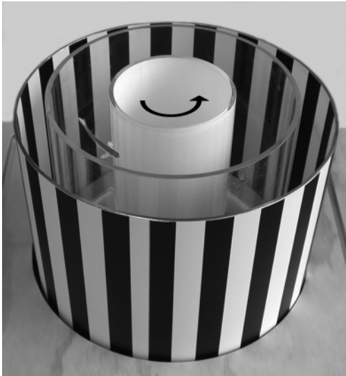
FIG. 4. Adult optomotor response (OMR). A single adult zebrafish is placed into a circular tank surrounded by a moving drum fitted with black and white stripes. The fish will swim with the moving stripes.
