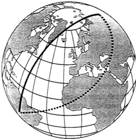
Fig. 2.7 Orthodrome (great-circle) and loxodrome (constant-angle) courses drawn on the surface of the globe. Solid line, orthodrome; dotted line, loxodrome.
